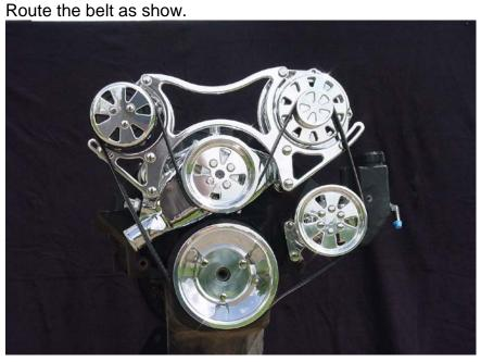
Pull adequate tension on the belts and tighten bolts.
