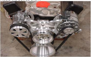
Pull adequate tension on the belt and tighten bolts.
