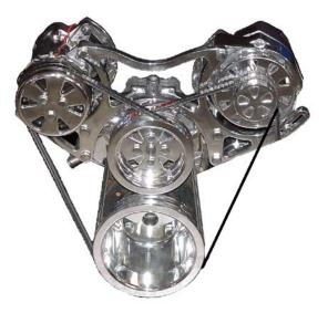
First using the 15445 belt, route it on the grooves in the back of the Water pump and Crank pulleys, then around the Alternator.
